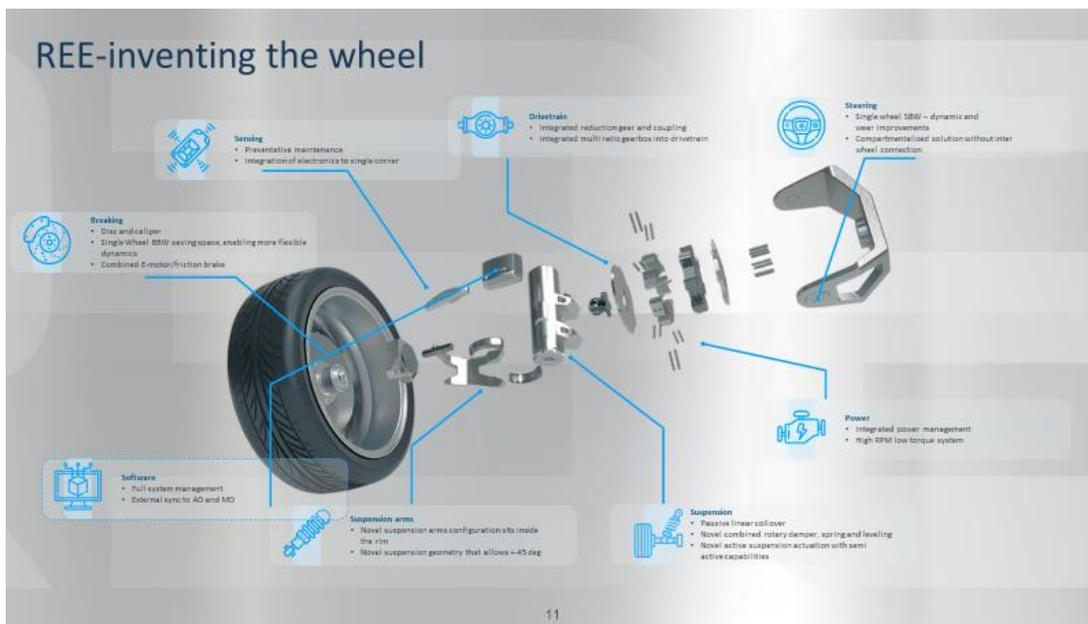
REE's unique approach strategically places the motor, steering, suspension, drivetrain, sensing, brakes, thermal systems, and electronics into the wheel, creating a truly flat platform. This design provides a low center of gravity to maximize efficiency and supports the vehicle's agility and stability. REE's innovation drastically reduces a vehicle's footprint and weight and improves both energy efficiency and performance – aspects crucial to the electric and autonomous vehicle revolution.
